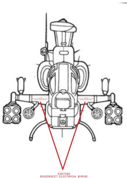
CAUTION DISCONNECT ELECTRICAL WIRING BEFORE REMOVING WING
